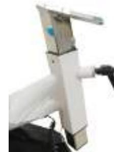
Loosen the locking bolt and adjust the height. Then, fasten the locking bolt again.
